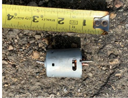
Figure 5: Washer pump motor
