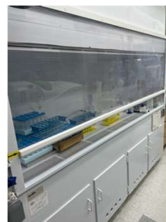
Chemical Fume Hood
